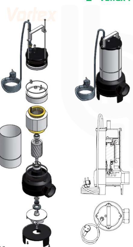
The range **Vortex F** is designed for pumping of sewage with suspended solids, it is ideal for installation with guide rain.
